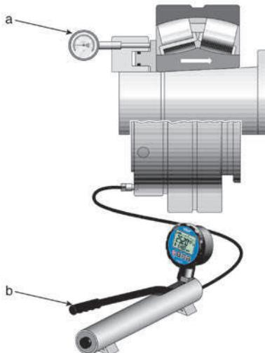
Figure 9. Dial indicator and hydraulic pump.
