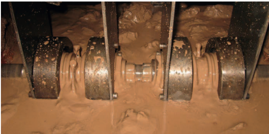
Mudslurry test rig
