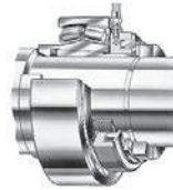
Figure 8. HMV nut and stop ring in position to press loose an adapter sleeve
