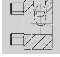
Frictionally engaged, backlash-free shaft-hub-connection for radial assembly of couplings. Transmittable torques depending on the bore diameter. (Only for ATEX category 3)
