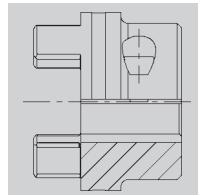
Positive power transmission with additional frictional tightness. The frictional tightness avoids or reduces reversal backlash. Surface pressure of the keyway connection is reduced.
