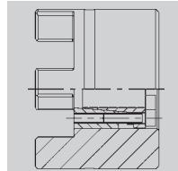
Frictionally engaged, backlash-free shaft-hub-connection for transmission of larger torques. Largest clamping set possible depends on the hub collar diameter. Clamping set screw fitting possible both internally and externally. For details of calculation please see CLAMPEX® catalogue.
