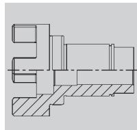
Special lengthened hub/shaft with integrated cams.
