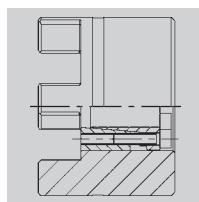
Frictionally engaged, backlash-free shaft-hub-connection for transmission of larger torques. Largest clamping set possible depends on the hub collar diameter. Clamping set screw fitting possible both internally and externally. For details of calculation please see CLAMPEX® catalogue.
