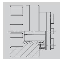
Frictionally engaged, backlash-free shaft-hub-connection for transmission of average torques.
