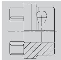
Frictionally engaged, backlash-free shaft-hub-connection. Transmittable torques depend on the bore diameter (page 34). (Only for ATEX category 3)
