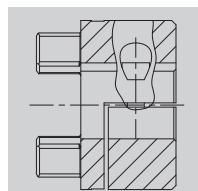
Positive power transmission with additional positive locking for radial assembly of couplings. Positive locking prevents or reduces reversing backlash, respectively. Surface pressure of the feather key connection is reduced.
