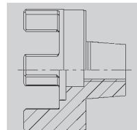
Special hub with external taper as a frictionally engaged connection.
