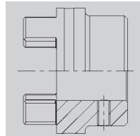
Positive torque transmission for connections pressed or glued in. (No ATEX release)
