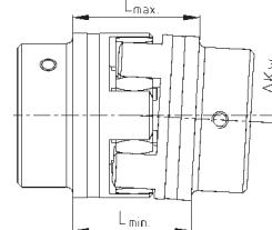
$$\Delta K_w [\text{mm}] = L_{\max} - L_{\min}$$
