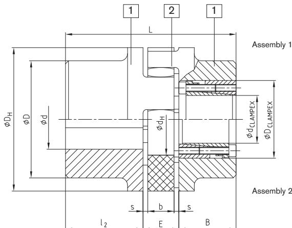
ROTEX® type No. 001 with clamping set CLAMPEX® KTR 200
