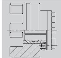
Frictionally engaged, backlash-free shaft-hub-connection for transmission of average torques.
