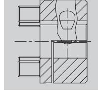
Positive power transmission with additional frictionally engaged operation for radial assembly of couplings. The frictionally engaged operation prevents or reduces reversing backlash, respectively. Surface pressure of the feather key connection is reduced.
