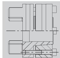
Design equal to 6.0, but clamping screws to be fitted externally. Suitable, for example, for disassembly of radial spacer tubes (special design).
