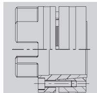
Integrated frictionally engaged shaft-hub-connection for transmission of higher torques. Screw fitting on elastomer side. For details about torques and dimensions see on page 33. Suitable for high speeds.
