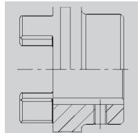
Positive power transmission; permissible torque depends on the permissible surface pressure. Not suitable for backlash-free power transmission for heavily reversing operation.
